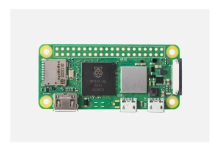
Raspberry Pi Zero 2 W is the latest product in our most affordable range of single-board computers. The successor to the breakthrough Raspberry Pi Zero W, Raspberry Pi Zero 2 W is a form factor—compatible drop-in replacement for the original board.
