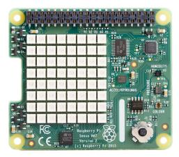
The Raspberry Pi Sense HAT gives your Raspberry Pi an array of sensing capabilities. The on-board sensors allow you to monitor pressure, humidity, temperature, colour, orientation, and movement. The bright 8x8 RGB LED matrix allows you to visualise data from the sensors, and the five-button joystick lets users interact with your projects.
