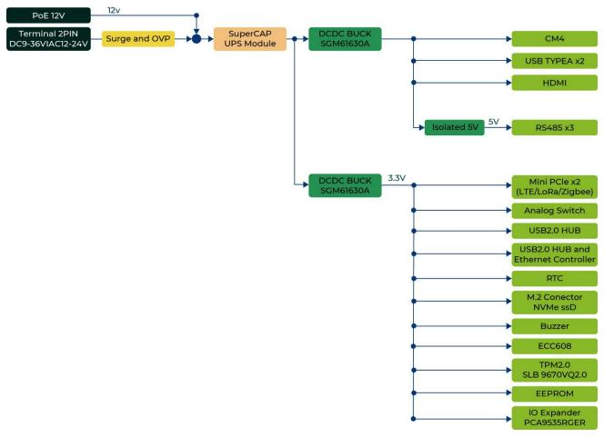
The reComputer R1000 supports three power supply options: AC, DC terminal and PoE port. By default, the reComputer R1000 is powered through the AC/DC terminal (Official regional power adapter SKU:110061505/110061506), while the PoE power supply(PoE module, SKU:110991925) is optional. This provides flexibility in power supply selection and allows for easy integration with various power sources.
