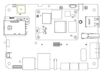
The reComputer R1000 features an active buzzer, which can be used for various purposes such as alarm and event notifications. The buzzer is controlled through GPIO21 to CM4.
