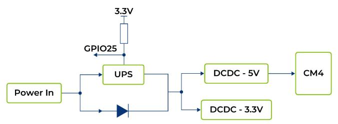
The UPS is 7F, which operates in series. The UPS module is positioned between the DC5V and CM4 components, with a G PIO signal utilized to alert the CPU in the event of a power loss from the 5V supply. Upon receiving this signal, the CPU ex ecutes an urgent script before the super capacitor's energy is depleted, initiating a "\$ shutdown" command.
