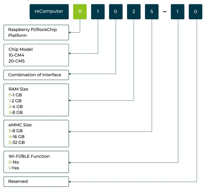
For example, the naming of 4GB RAM and 32GB eMMC CM4 module with Wi-Fi and BLE function tailored for smart building is reComputer R1025-10.
